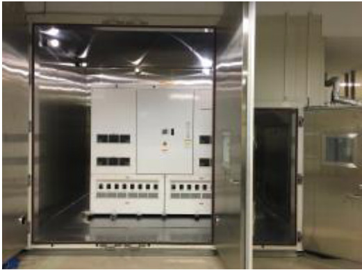
PV Inverter: High Temperature High Humidity Test
